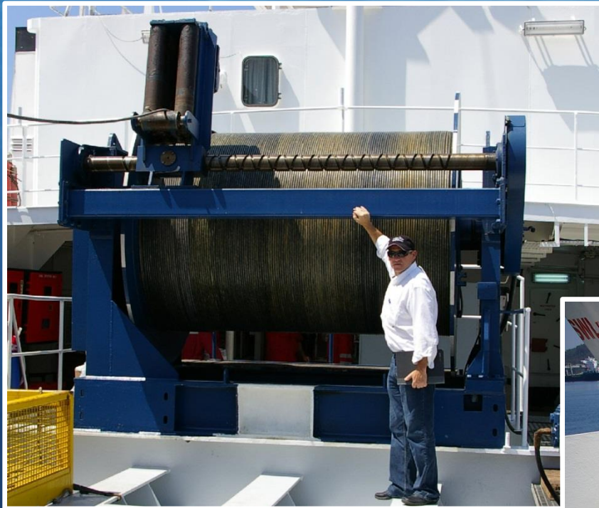
Deep Tow Winch with 10,000 meters of tow cable
